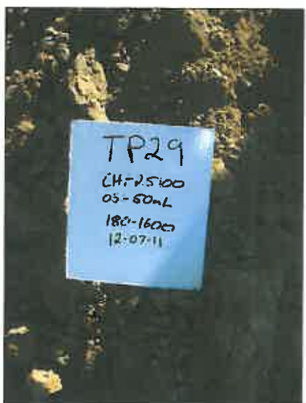
Excavated material from 0.18-1.6m
