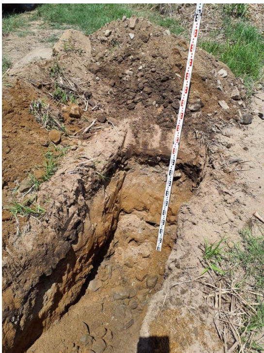
TPL-12 - 1 Test pit excavation - sidewall collapse occurring below 0.7 m below ground level
