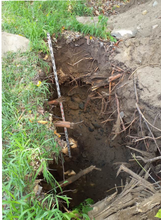
TPL-11-1 Test pit excavation - sidewall collapse occurring below 3.0 m below ground level
