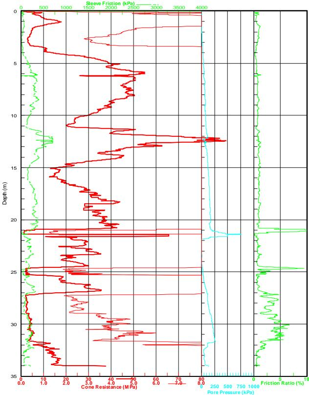
Tested By: SW & GB Test Date: 23/04/2003 IGS No: 1275 Job No: 0304-23 Tested in accordance with AS 1289.6.5.1-1999. Page No: 1 of 1
