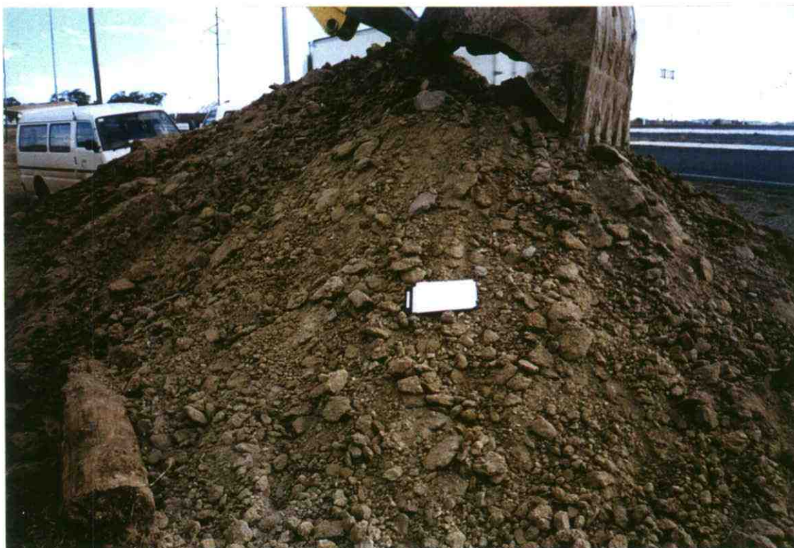
Plate 20: Excavated material from TP7
