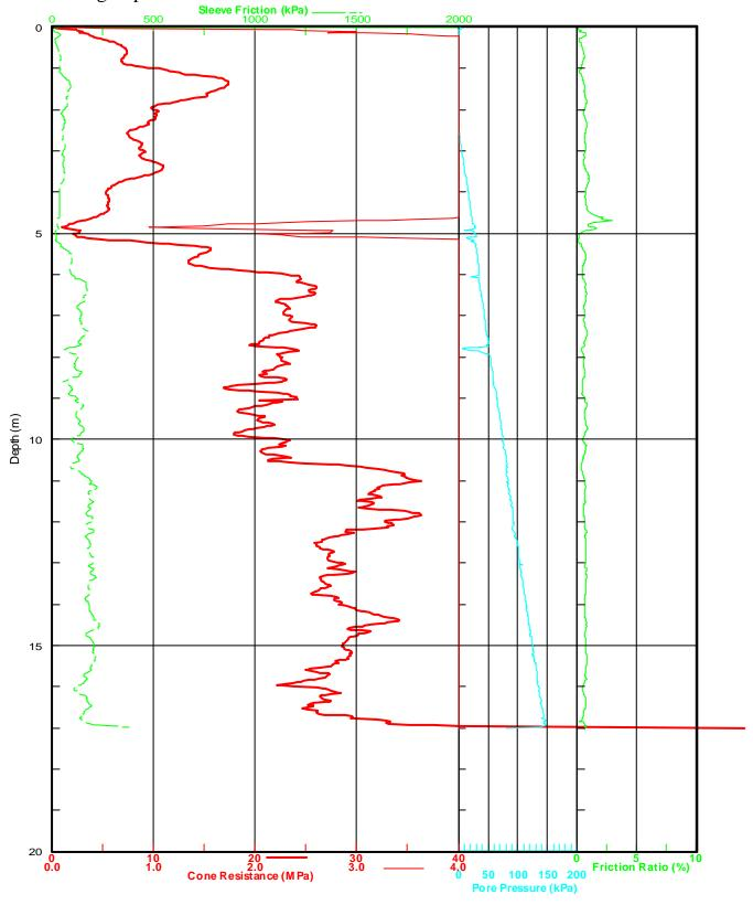
Tested By: SW & GB Test Date: 10/05/2003 IGS No: 1311 Job No: 0805-08 Tested in accordance with AS 1289.6.5.1-1999.
