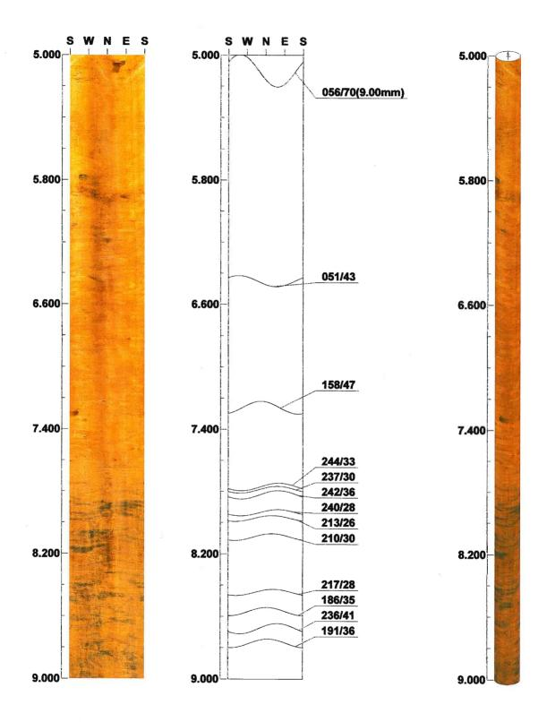
Bore hole No.: C-57 Azimuth: 0 Inclination: -90
