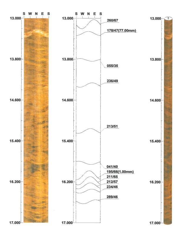
Bore hole No.: C-57 Azimuth: 0 Inclination: -90
