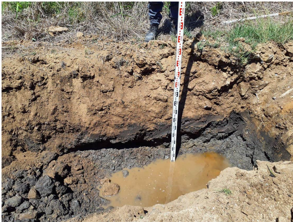
TPL-10-1 - Test pit excavation - sidewall collapse occurring below 0.9 m below ground level
