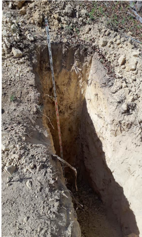
TPL-16-1 Test pit excavation - sidewall collapse occurring below 2.7 m below ground level
