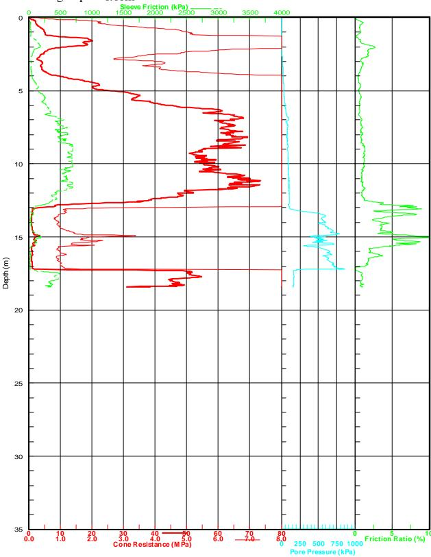
Tested By: SW & GB Test Date: 07/06/2003 IGS No: 1341 Job No: 0806-04 Tested in accordance with AS 1289.6.5.1 -1999. Page No: 1 of 1
