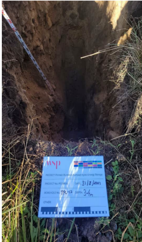
TPL-13 - 1 Test pit excavation
