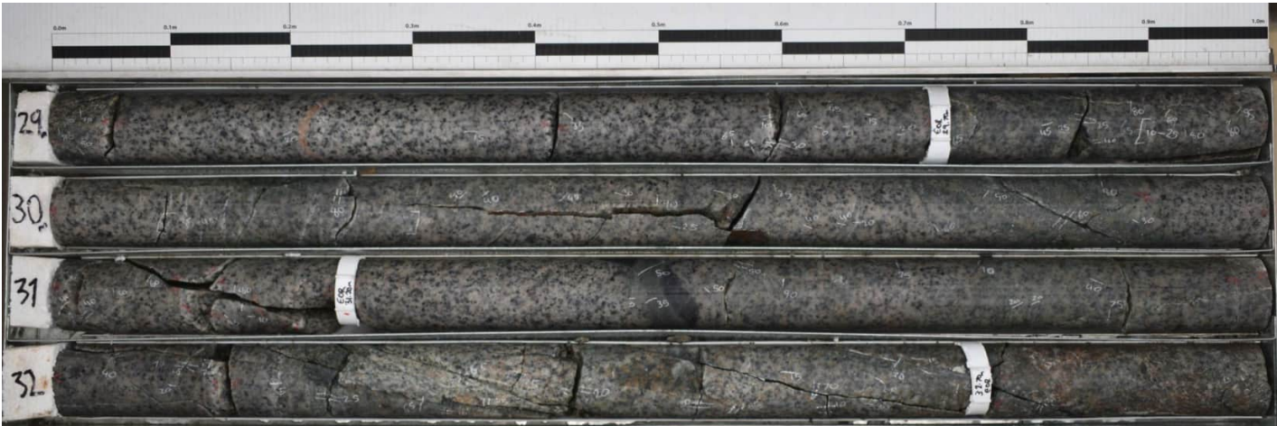
PointID : BGL-05 Depth Range: 29.00 - 33.00 m
